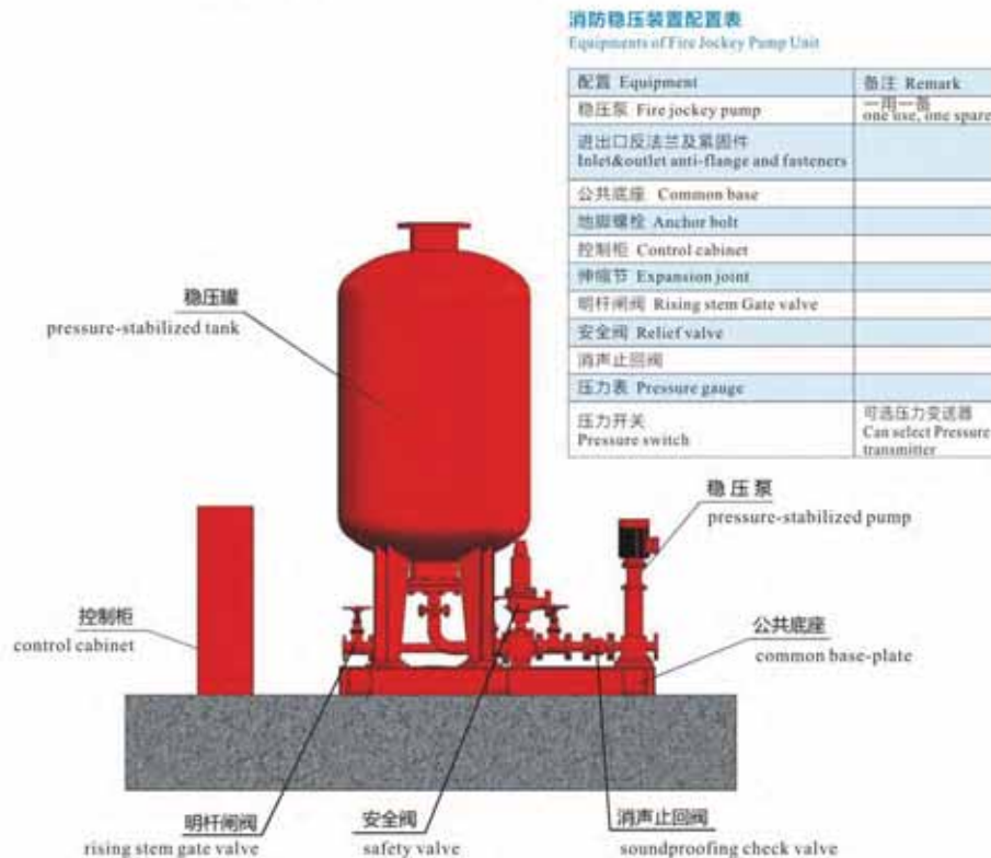
(Figure 4) Fire voltage stabilizing device schematic diagram (Apply To Vertical Fire Pump, Horizontal Fire Pump)
